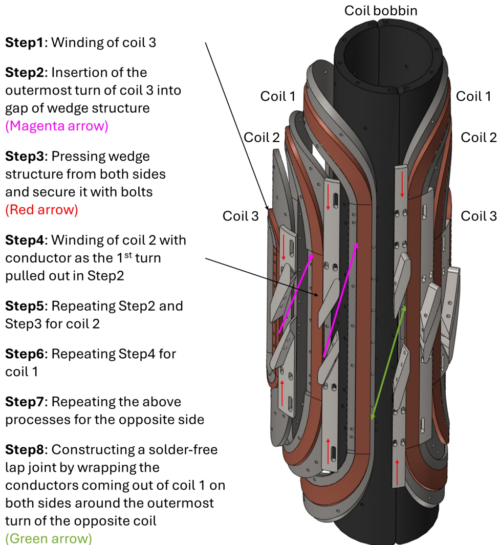
Figure 3.21: Overall summary of coil assembly process
